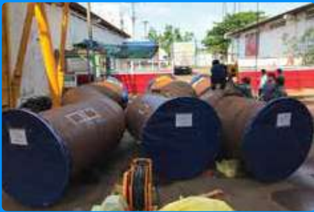
Flange and external rubber surface shall be in protection packaging for delivery.
