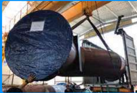
Flange and external rubber surface shall be in protection packaging for delivery.
