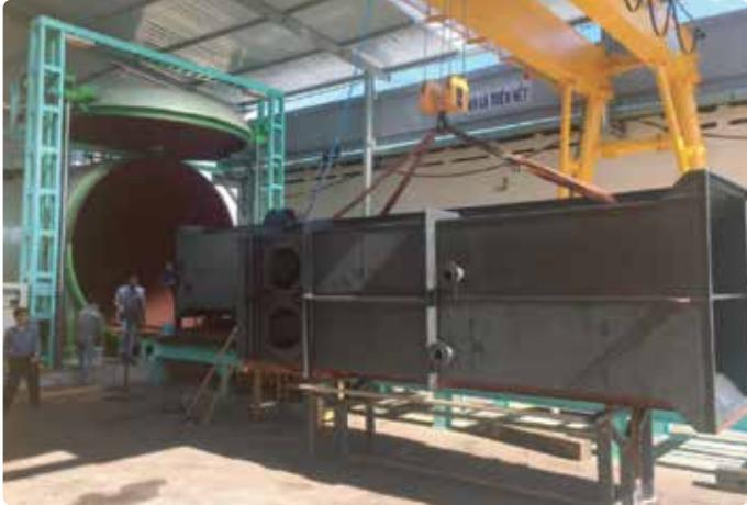
Both face rubber lining resin pickling tank
