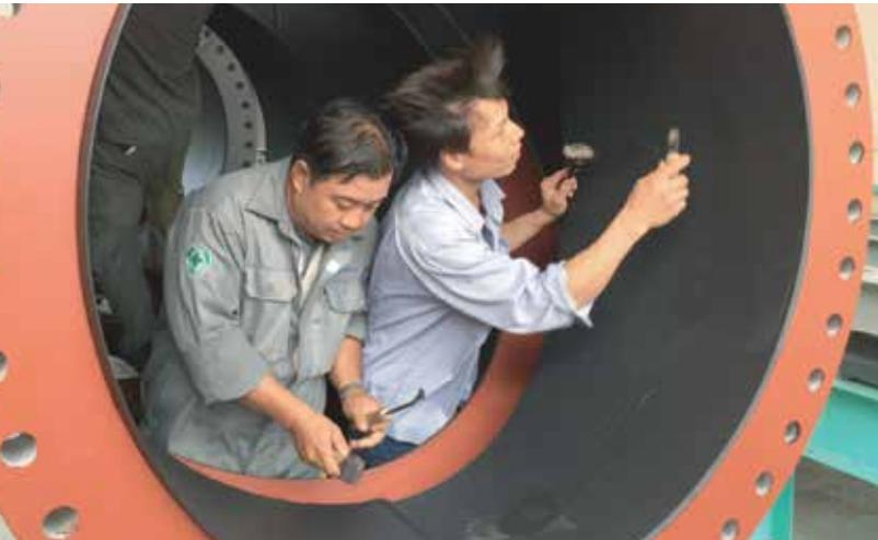
Rubber sheets shall be firmly bonded to steel substrate after application of primer and adhesive. Lining is done by hand by our experienced staff for a durable finished product. After application of rubber sheets and proper vulcanizing, rubber lining provides rubber elasticity, superior strength and chemical resistance.
