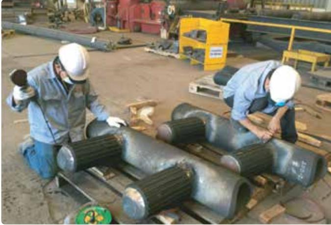
Finishing Neoprene Rubber lining for wind tower
