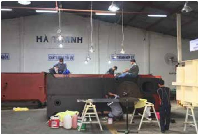
Both face tank Rubber lining at HT Shop
