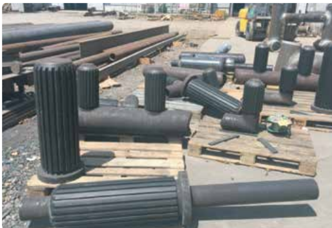
High quality 25mm Neoprene-lined rubber pre-erection in wind tower
