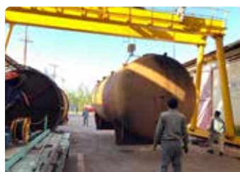
Gantry crane 10T
