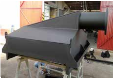
Cover / Roof of chemical tank
