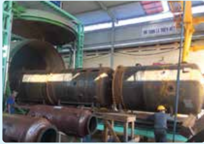
Vulcanizing autoclave (ID4m*12mL)
