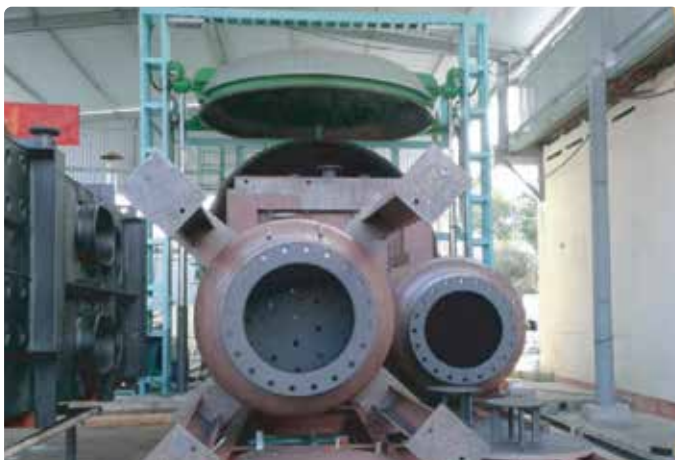
Finished vulcanization chemical vessel
