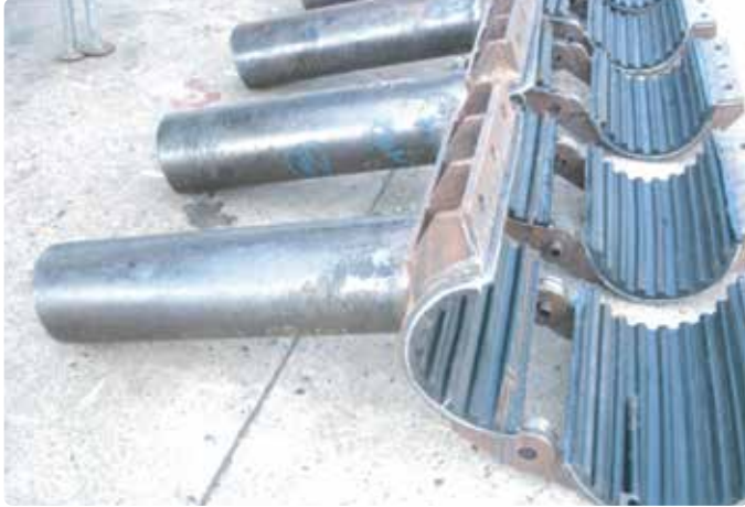
Riser clamps with Neoprene lining
