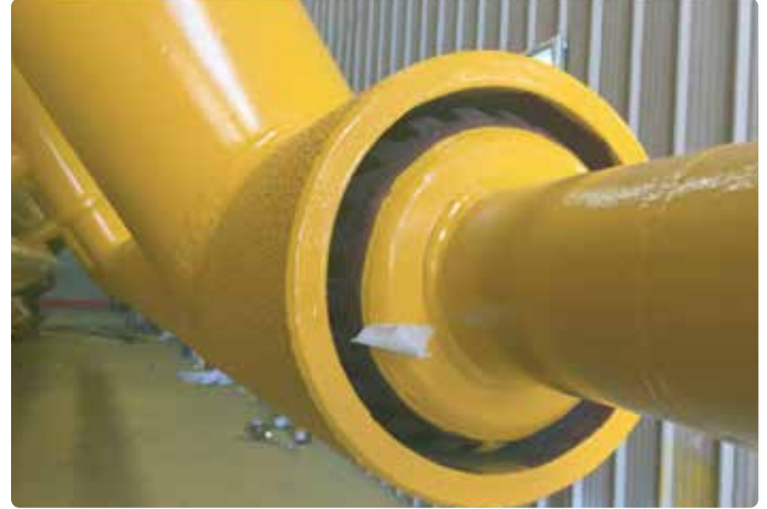
Neoprene Rubber lining for wind tower
