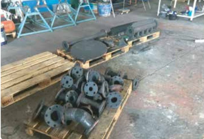
Lining pipe spool
