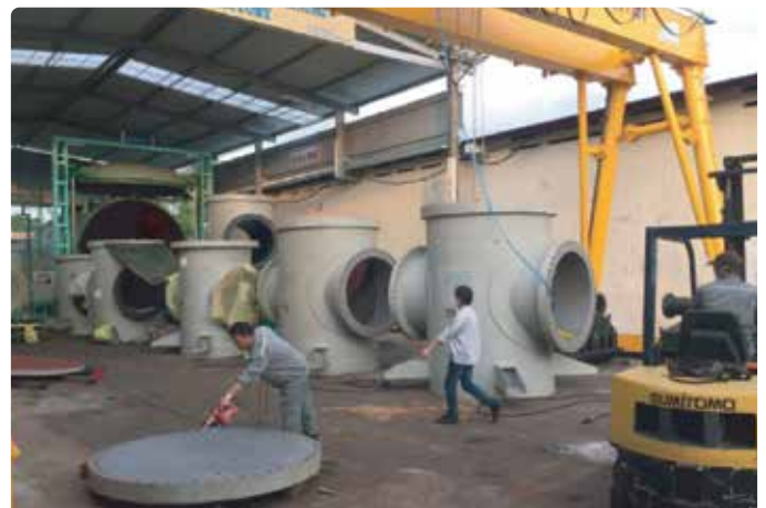
Rubber lining sea strainers equipment at shop
