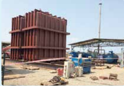
Open or direct steam curing
