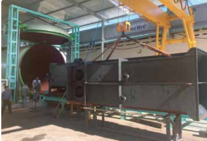
Both face rubber lining resin pickling tank
