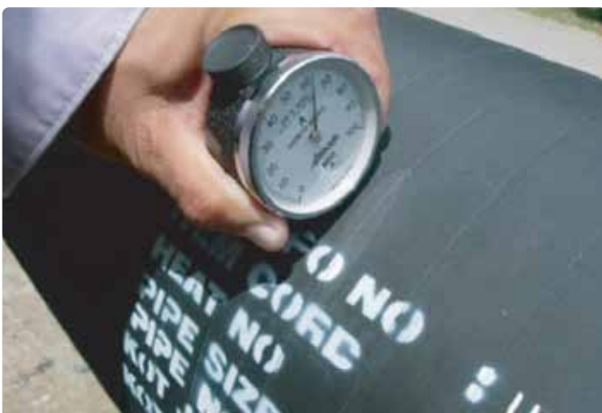
Checked with hardness tester
