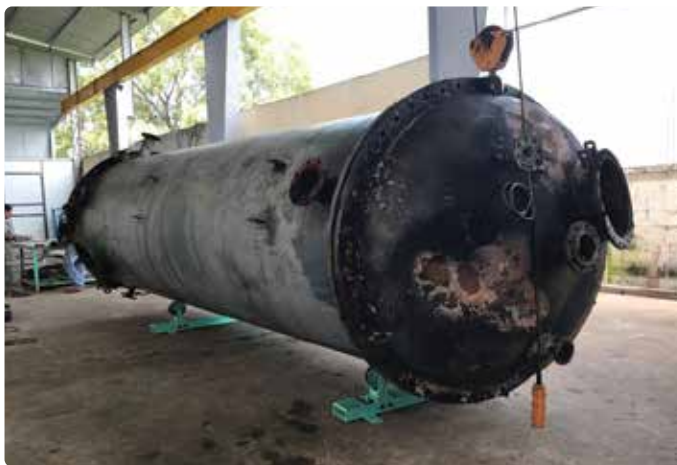
Replace old substrate after 18 years used
