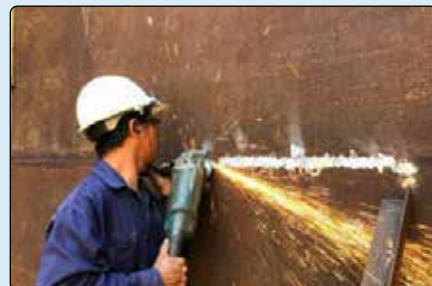
Fill or grinding not overlap-welded
