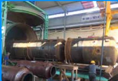
Vulcanizing autoclave (ID4m*12mL)
